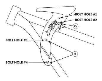
**STEP 6:** Insert the two Long Bolt Sets (**part H**) (or Extra Long Bolt Sets (**part** I) if your down tube is wide), into bolt holes #3 and #4. You can pivot the bottom of the Mainframe forward or backward to level the saddle.
