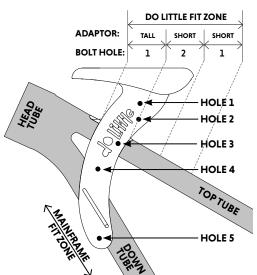
**STEP 4:** Attach the Adaptor. Position the chosen adaptor (part B or C) on the top tube by by feeding the Velcro Strap (part D) through the adaptor and around the top tube, ensuring it is tight. The Tall Adaptor (part C) has two options/holes for adjusting the height of the Mainframe. Use whichever hole suits your preference for fit.
