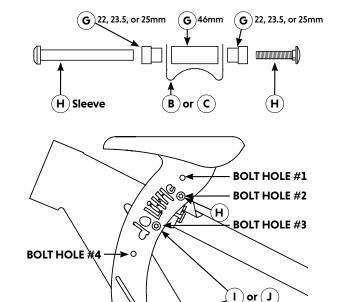
**STEP 8:** Check the Mainframe positioning and tighten the Short Bolt Set (**part H**) and Long Bolt Sets (**part I or J**) with the Multi Tool (**part K**). Test to be sure the Do Little Kids Bike Seat does not move.
